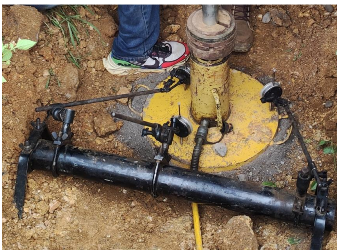
Figure 4. Reference beam used for plate load test is too near the bearing plate.
